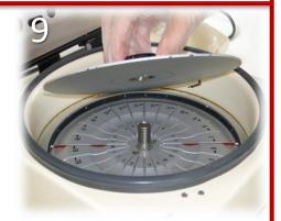
Screw the metal cover (plate) on firmly. Close and secure the centrifuge lid.
