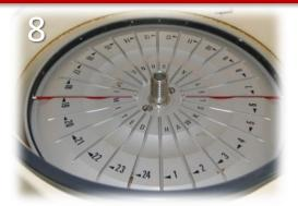
Fill 2 tubes and place them opposite each other in the centrifuge. This is to balance the centrifuge; every tube must have another tube opposite it. Place the plasticine plug end of the tube against the rubber (outer) edge to stop the contents spilling out when spun.
