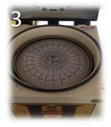
Check that the centrifuge is clean and free from debris or previous samples.
