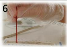
Make sure there is an area of the plasticine that is clear from previous holes. Place the capillary tube onto the plasticine then remove your index finger from the top. Having removed your finger then gently press the capillary tube into the plasticine and then withdraw the tube. Wipe the tube clean with a tissue.
