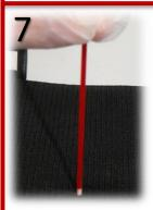
Check there is a sufficient plasticine plug. If not, then discard the capillary tube into a sharps bin and start again.
