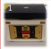
Switch on the centrifuge at the wall. Some centrifuges also have a switch on the machine. Open the lid – some centrifuges have a button while others have a catch.
